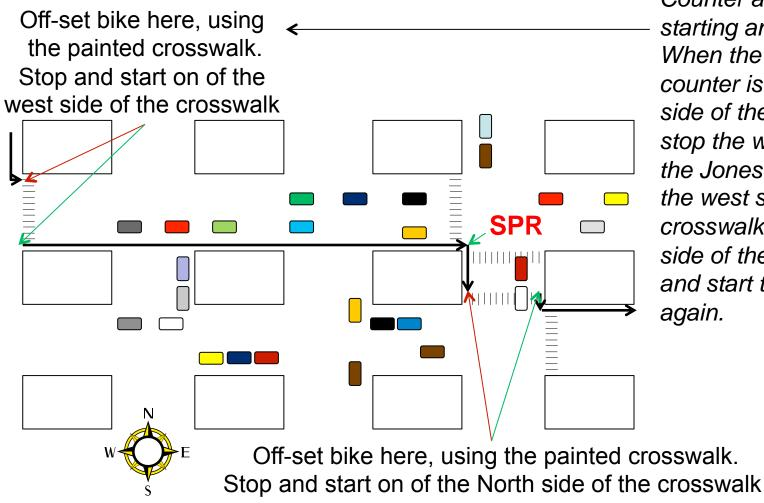
Use your Jones Counter as the point of starting and stopping. When the Jones counter is at the west side of the crosswalk, stop the wheel. Place the Jones counter on the west side of the crosswalk on the south side of the intersection and start the wheel again.
