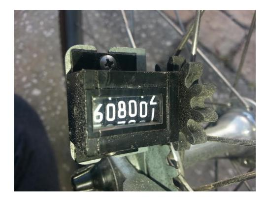
This Jones Counter is a 6 digit model. It currently reads 608002. I round up when writing the count at the end of my first calibration ride, but the Jones Counter is locked and will start the second calibration ride on the partial count as shown.
