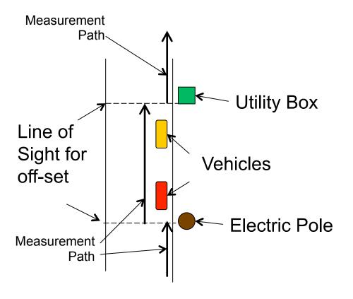
When off-setting, pick objects close to where you want to offset. Ride up to the objects, Line Jones Counter up with object, Lock your Brake, Move the Bike over, Ride as straight of a line as possible to the next object in the road, Line up your Jones Counter and Move bike back over. Continue on with measurement.
