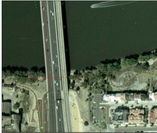
Figure 4. Loss of observations due to loss of sky visibility (Click for larger image).
