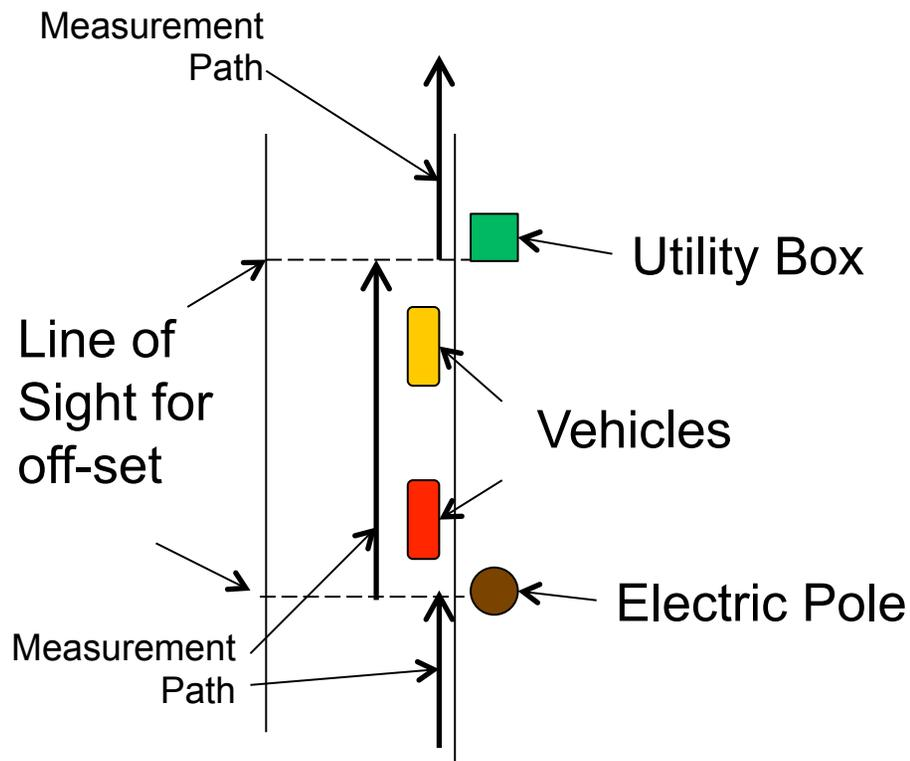
When off-setting, pick objects close to where you want to off-set. Ride up to the objects, Line Jones Counter up with object, Lock your Brake, Move the Bike over, Ride as straight of a line as possible to the next object in the road, Line up your Jones Counter and Move bike back over. Continue on with measurement.
