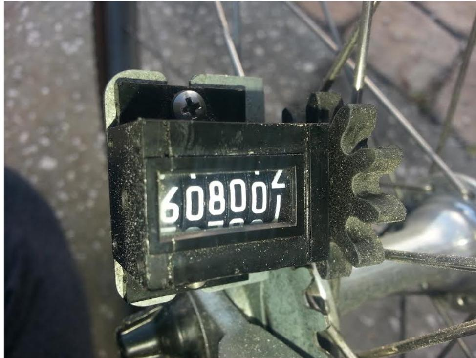
This Jones Counter is a 6 digit model. It currently reads 60800.4. I round up when writing the count at the end of my first calibration ride, but the Jones Counter is locked and will start the second calibration ride on the partial count as shown.
